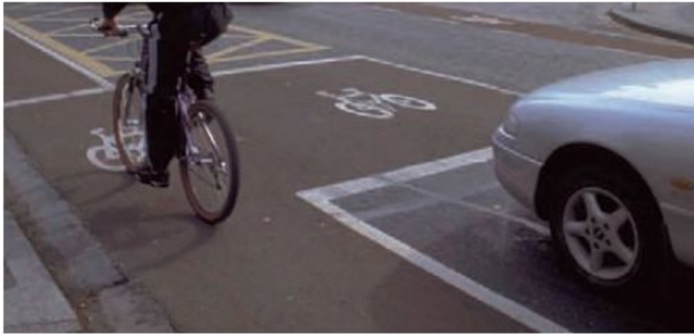
Figure 6.b Image from NCM showing advanced stacking location/advanced stop line for cyclists.
