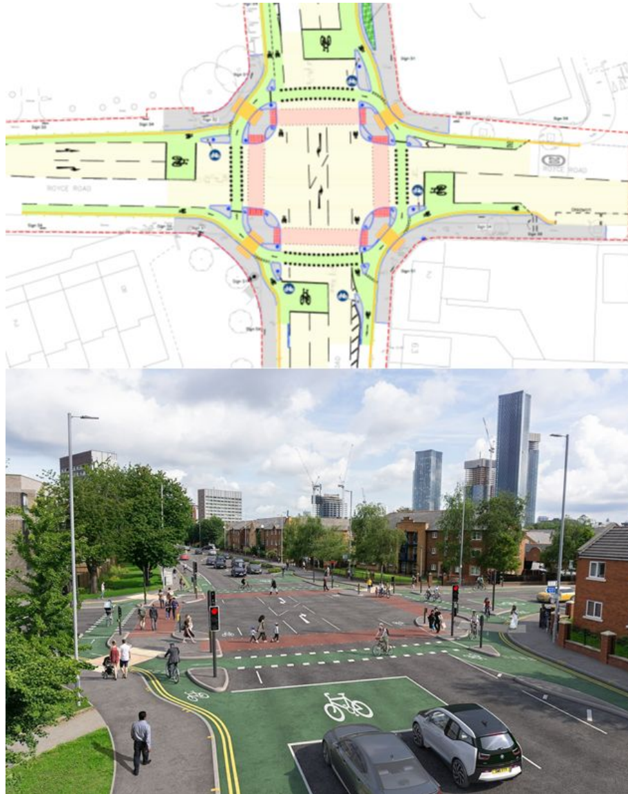
Figure 5.b Extract from Manchester to Chorlton Cycle Way scheme with design of protected cycling intersection.
