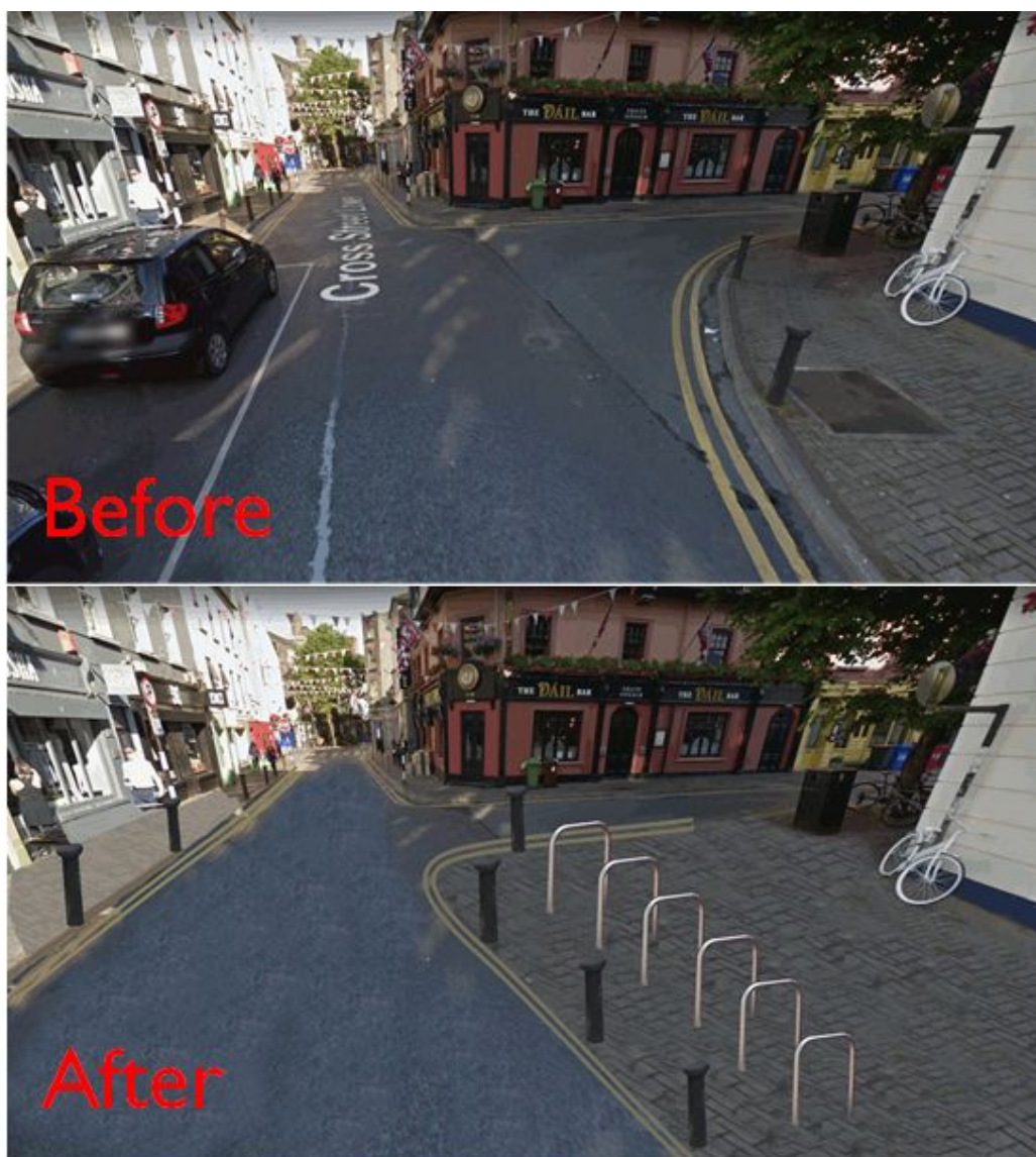
Figure 6.2 Mock-up design of a corner radius reduction at the junction of Cross Street and Middle Street. Further improvements could increase the aesthetic aspect of the street, in line with the Strategy.
