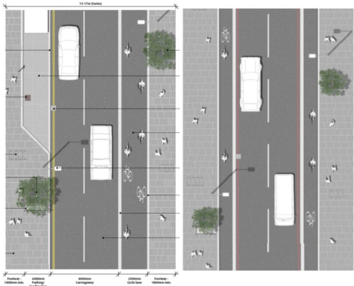
Figure 5.5 Street design in Strategy giving specifications for roadside segregated cycle lanes. The left panel indicates a bidirectional cycle lane of width 2.5m. It is unclear if the raised kerb is included in this width. The panel on the right indicates cycle lanes on either side of the roadway, of an unspecified width.
